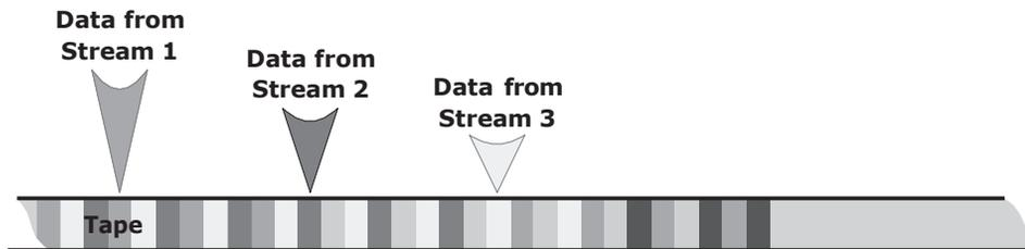
**Figure 10-16:** Multiple streams on tape media
