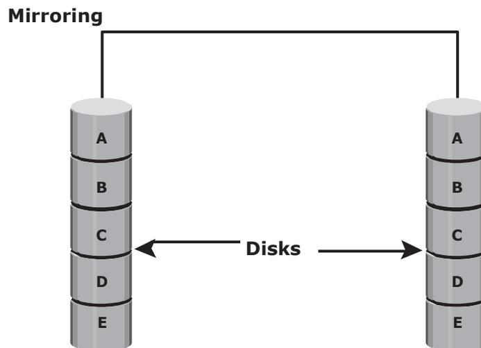
Figure 3-3: Mirrored disks in an array
