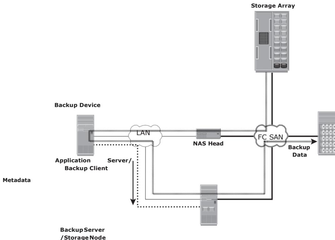
Figure 10-11: Server-based backup in a NAS environment
