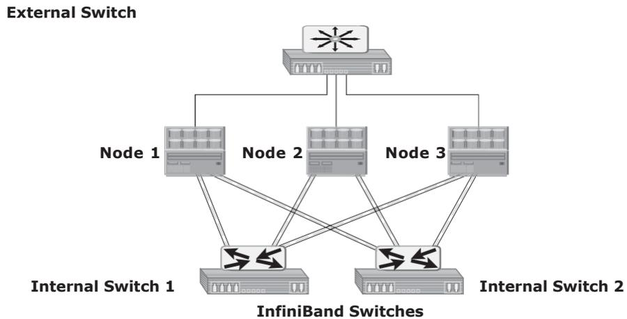
Figure 7-7: Scale-out NAS with dual internal and single external networks
