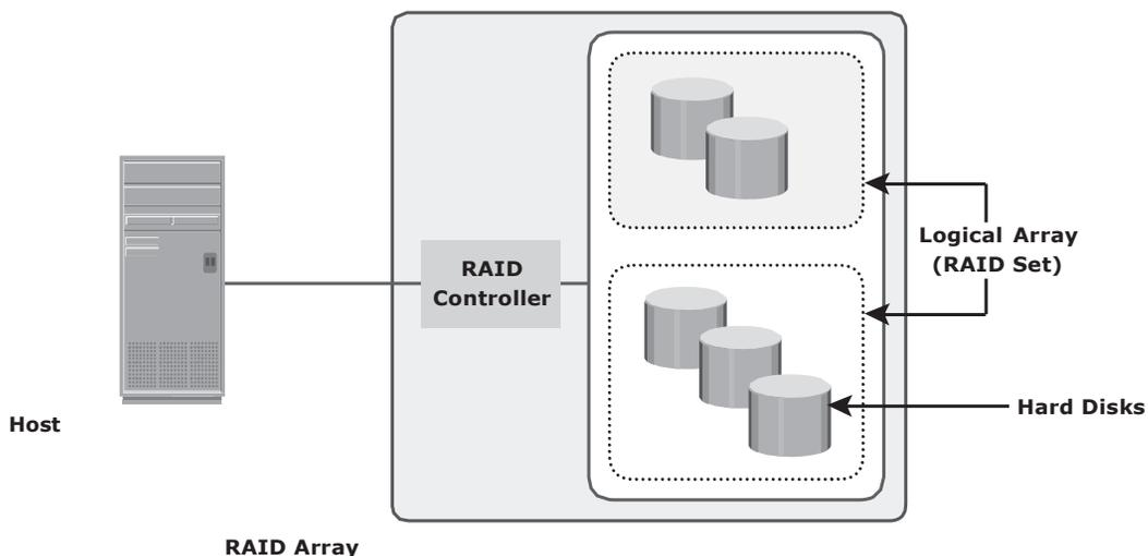
Figure 3-1: Components of a RAID array
