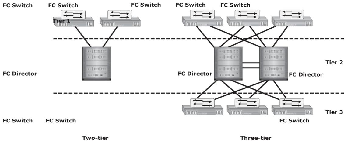
Figure 5-9: Tiered structure of Fibre Channel switched fabric
