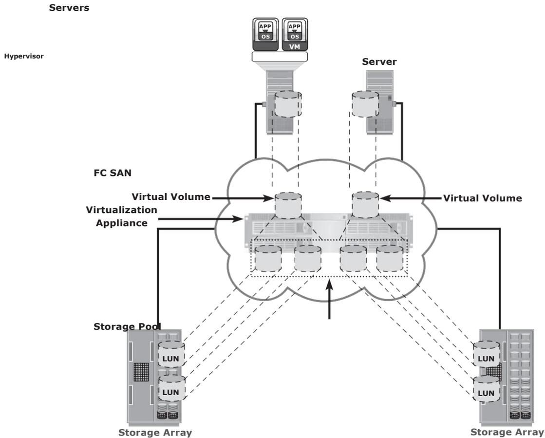
**Figure 5-24:** Block-level storage virtualization
