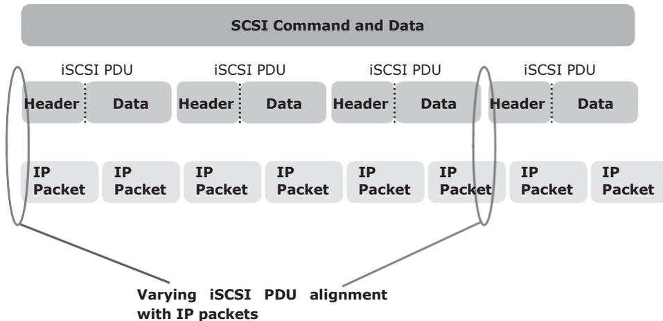
Figure 6-5: Alignment of iSCSI PDUs with IP packets
