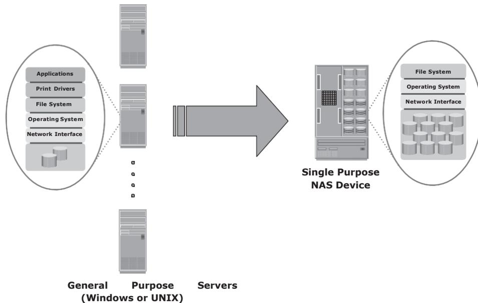
Figure 7-1: General purpose server versus NAS device
