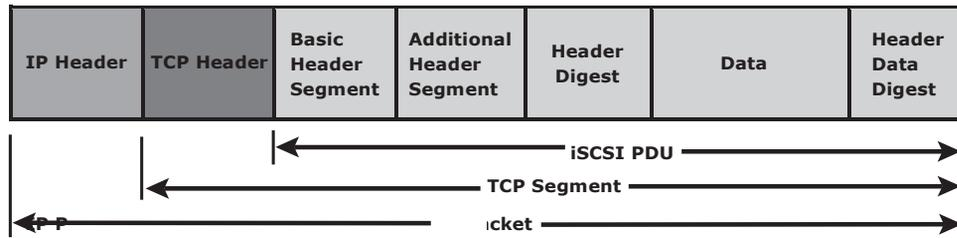
Figure 6-4: iSCSI PDU encapsulated in an IP packet
