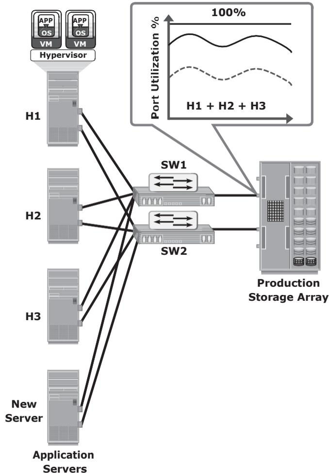
Figure 15-4: Monitoring array port utilization
