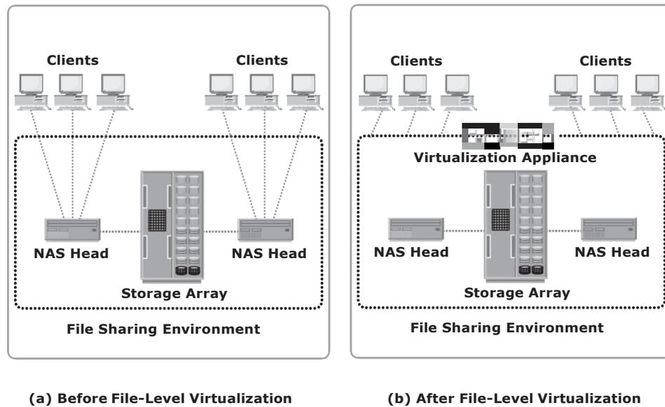
Figure 7-9: File-serving environment before and after file-level virtualization
