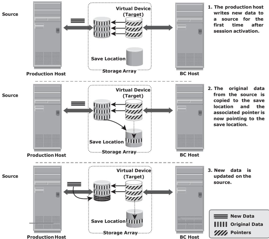
Figure 11-12: Pointer-based virtual replication — write to source
