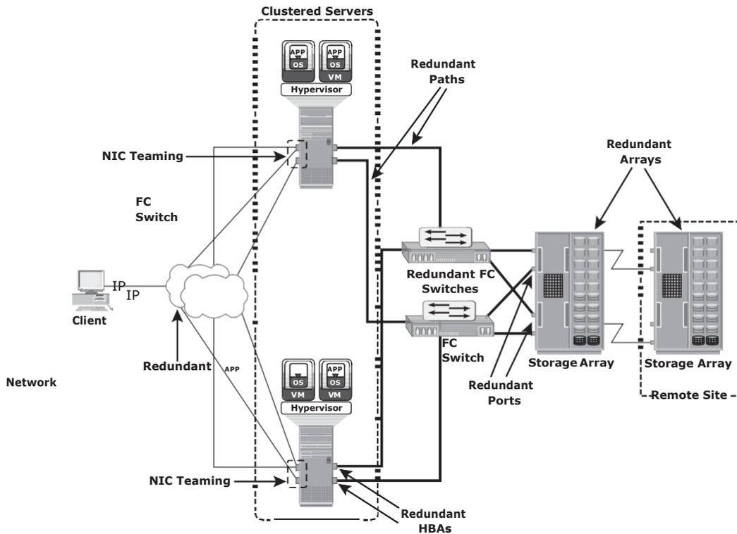
Figure 9-6: Resolving single points of failure
