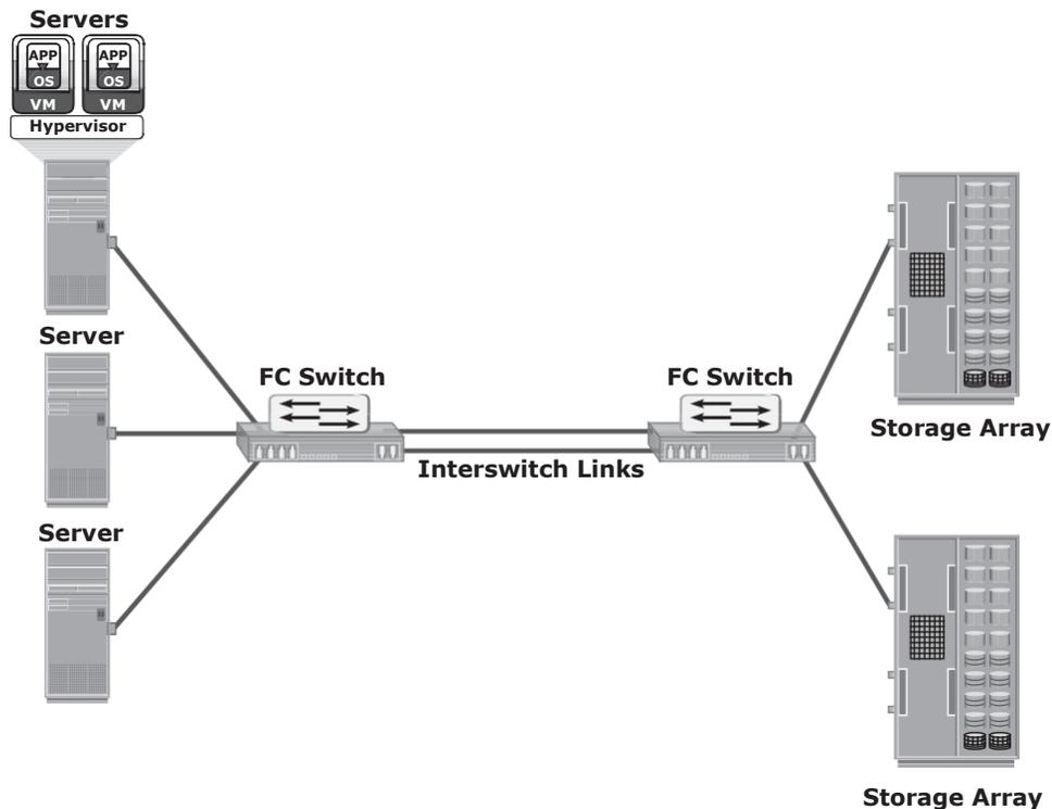
Figure 5-8: Fibre Channel switched fabric
