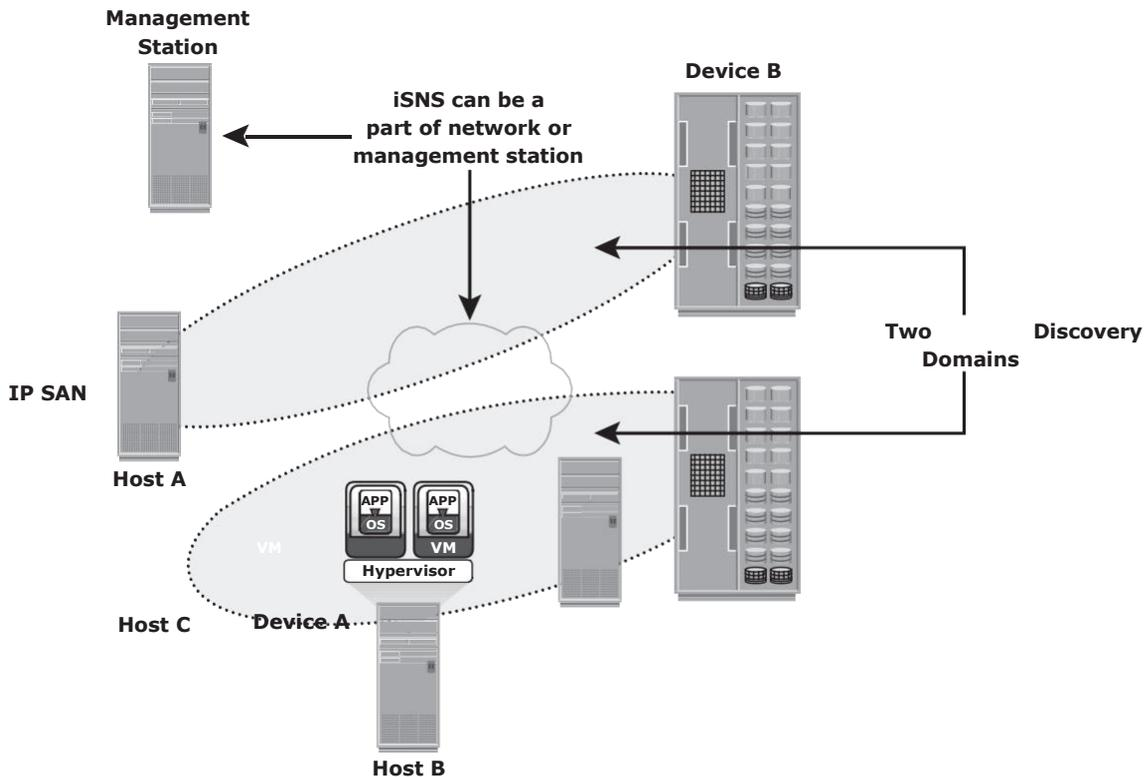
Figure 14-11: Securing IPSAN with iSNS discovery domains
