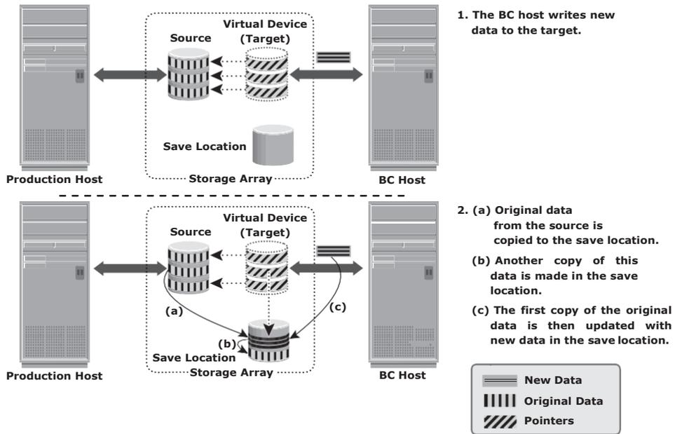
Figure 11-13: Pointer-based virtual replication — write to target
