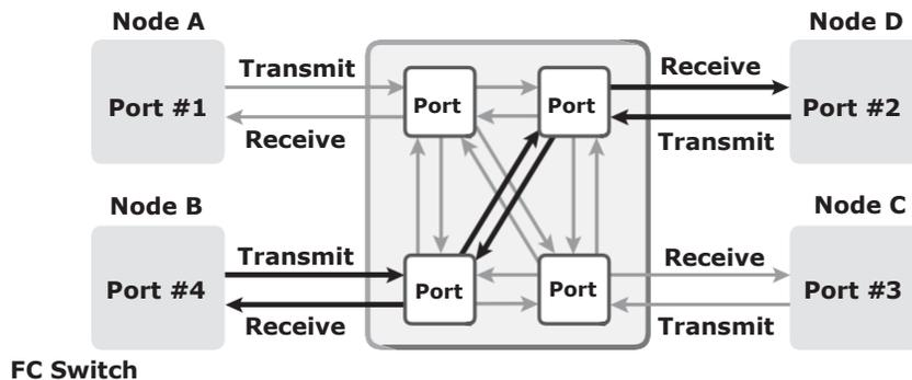
Figure 5-10: Data transmission in Fibre Channel switched fabric
