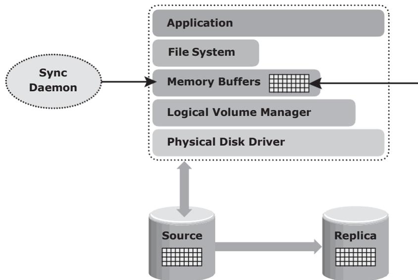
**Figure 11-1:** Flushing the file system buffer
